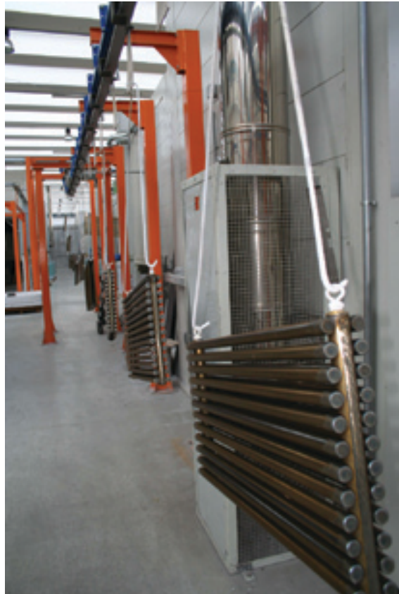
3 - Exit of radiators after drying and before entering the booth.
