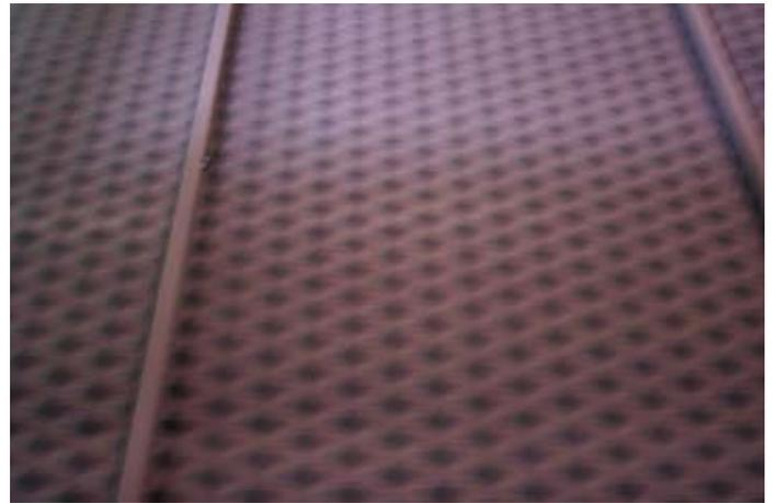
6a and 6b - An embossed grille before and after powder coating. Note the perfect coverage of the surfaces, even in the dips between the embossed parts, reached thanks to Atimix.
