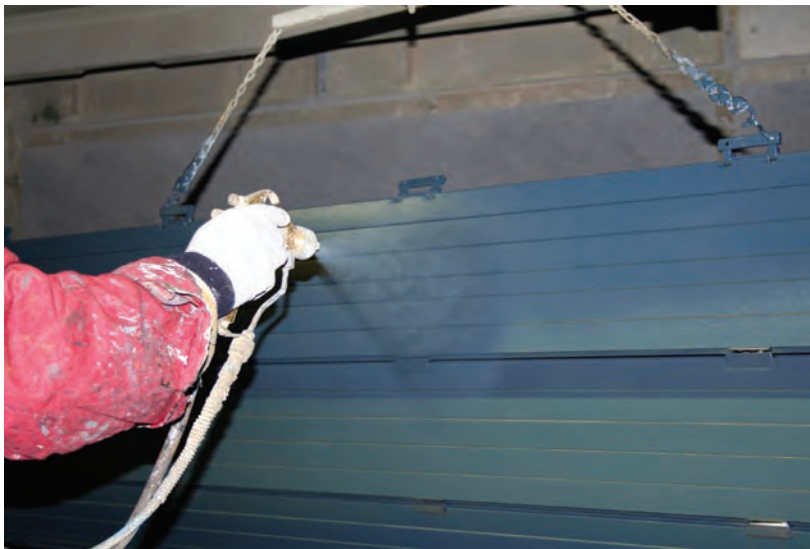
6 - The gun that sprays the water-based paint onto the leaves of the shutter: we can see that the overspray is reduced to a minimum and also we can note the precision of the direction of the paint, which is not deviated by disturbing electrostatic charges.
