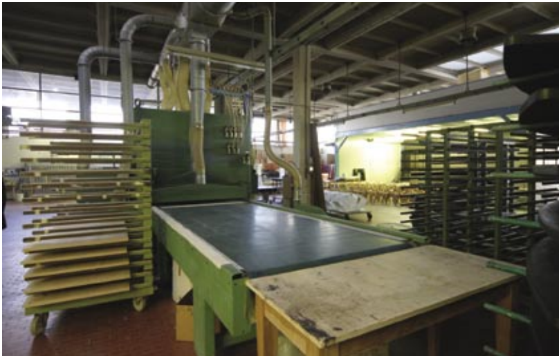
6 and 7 – The sanding operations can be done automatically or manually in the case of complex shapes.
