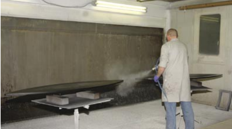
8 – The application of the finish on table tops.
