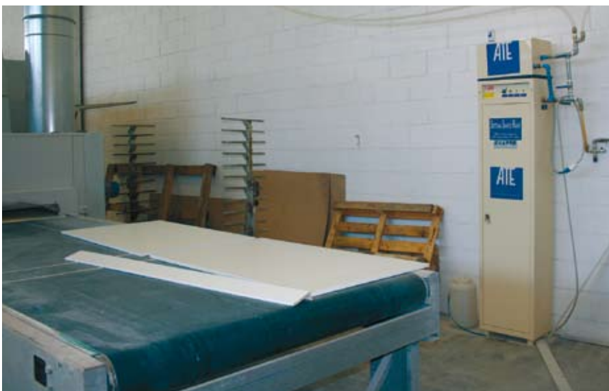
5 – The SimplePaint double column equipment that treats the application air of the automated system and the manual booth.
